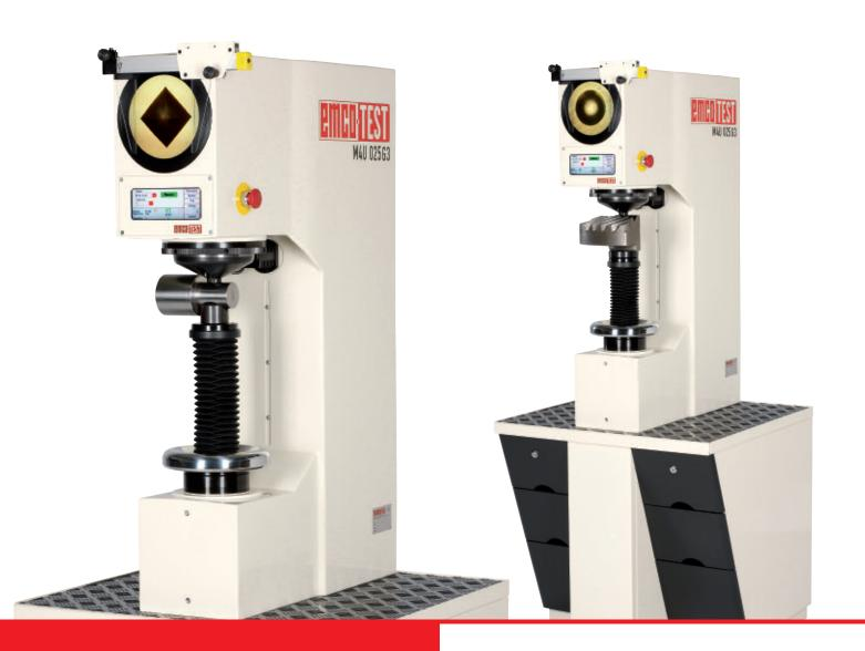
M4U 025/075 G3 M4U 250/750 G3 Universal hardness testing machines of the 3<sup>rd</sup> generation
