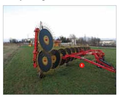
For transfers a hydraulic device allows the first two front finger wheels to be raised, reducing the rake length and making the machine more compact.
