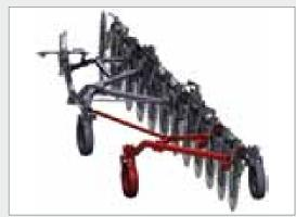
For optimal stability of the rear chassis in intensive conditions, for harvesting heavy forage and/or straw, a 5th wheel kit for additional support is available. This provides for the possible mounting of a further directional wheel (the 5th) in the rear left part of the rake.
