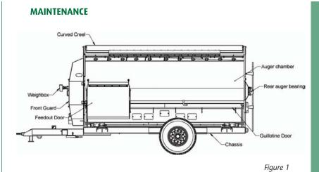
A properly operated and maintained Keenan mixer will give years of trouble free operation. **Regular maintenance of the machine is essential both for long machine life and to meet warranty requirements.** Refer to instructions in maintenance section of this manual. Weekly cleaning of machine is advised to prevent corrosion to the mixer body from old feed.
