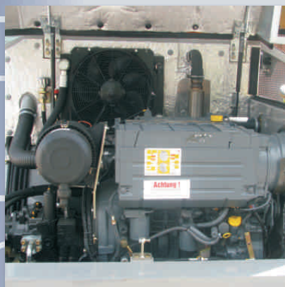
Extremely good accessibility for inspection and maintenance work due to the GFK engine cover that can be opened widely
