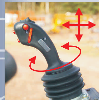
Electro-hydraulic servo control via multifunctional joystick. On TSL 855: swivel function by turning the joystick.
