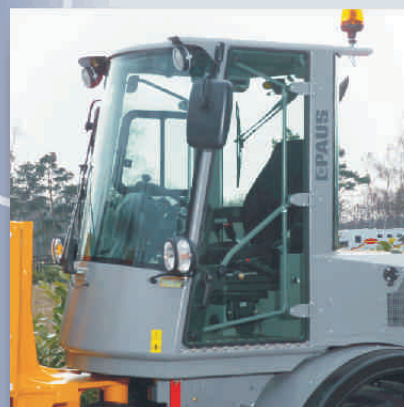
Plane entrance on both sides, control device foldable to the back, ergonomically designed joystick, orthopaedic comfortable seat with safety belt and disc support
