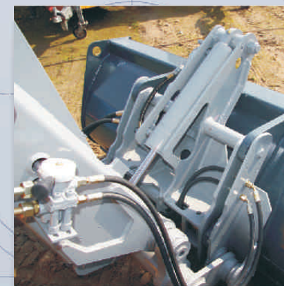
PAUS standard: hydraulic quick-change device for many attachments
