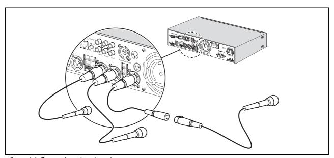
figure 4.4: Connecting microphone inputs
