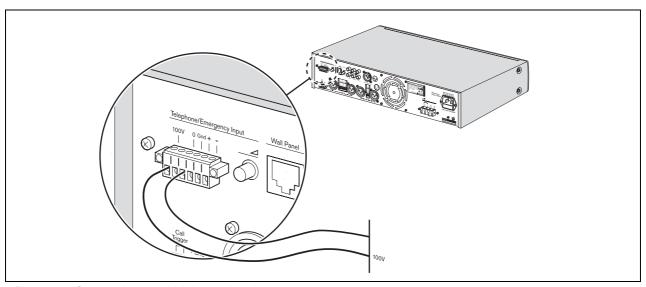
figure 4.5: Connecting 100 Volt input signal
