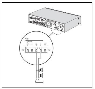
figure 4.10: Connecting speakers
