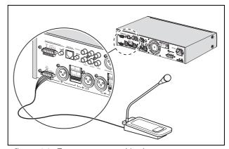
figure 4.3: Euro connector with trigger
