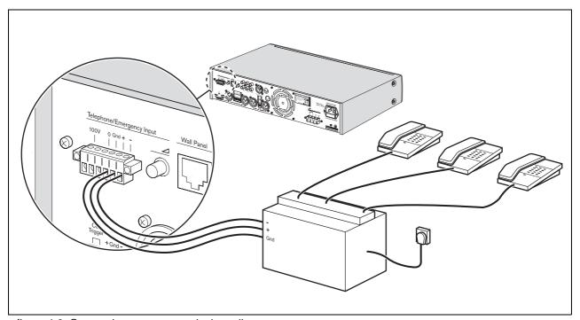
figure 4.6: Connecting emergency telephone lines
