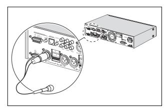
figure 4.2: XLR connector with trigger
