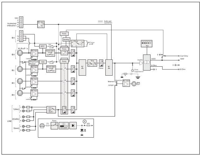
figure 2.1: Schematic overview of the Plena Mixer Amplifier
