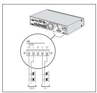
figure 4.9: Connecting speakers
