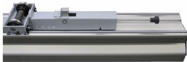
Fig. 5-28: Installing the middle carriage
