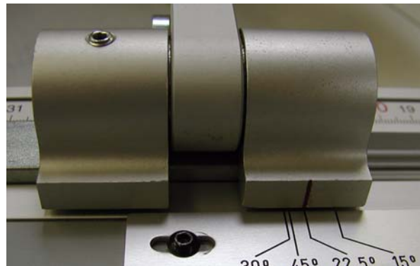
Fig. 6-126: Adjusting the fence stop
