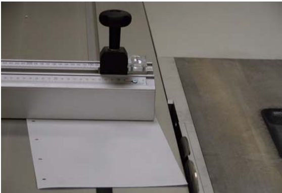
Fig. 5-48: Checking the cross-slide height
