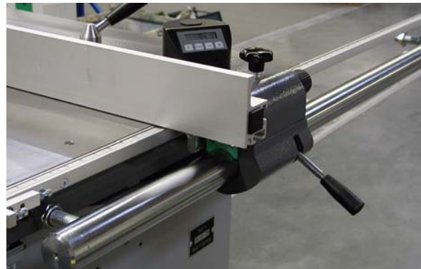
Fig. 5-8: Installing the rip fence
