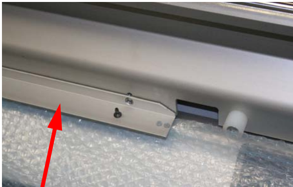
Fig. 5-33: Bracket on the bottom carriage
