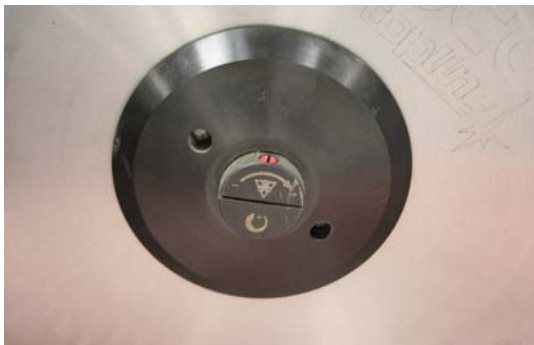
Fig. 6-26: Changing the saw blade
