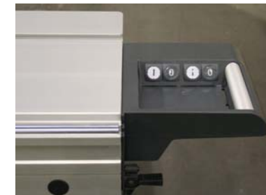
Fig. 6-24: Switches for saw drives, DRW
