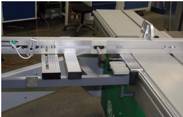
Fig. 5-15: Installing the WGA_LD
