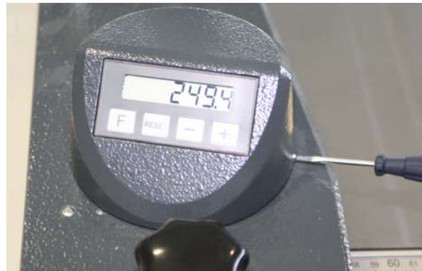
Fig. 6-137: Release the clamping screws
