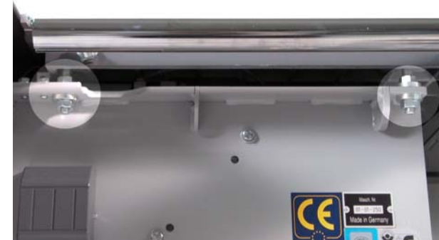
Fig. 5-46: Adjusting the main table
