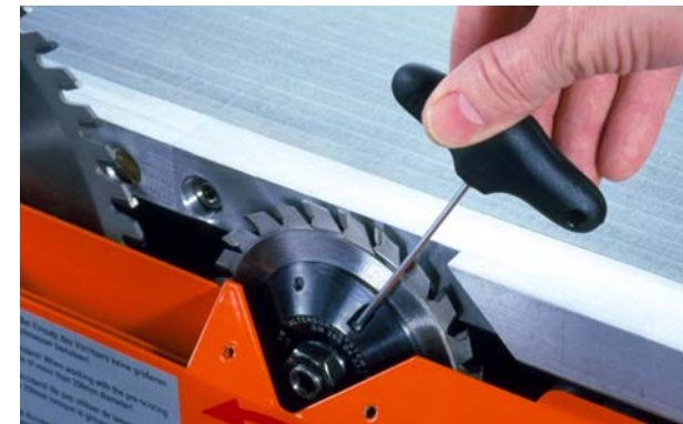
Fig. 6-112: Releasing the clamping screw
