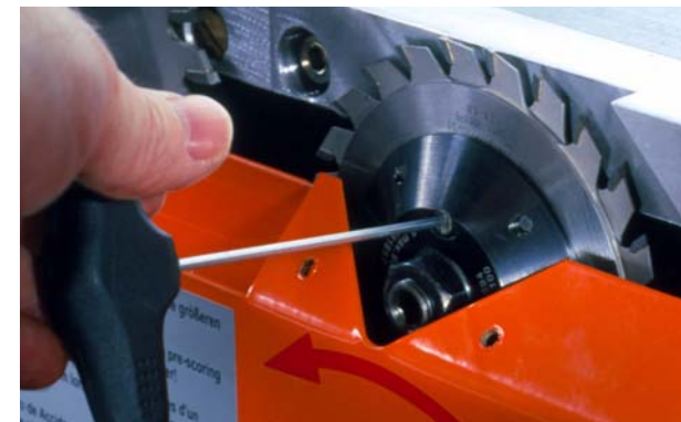
Fig. 6-113: Adjusting the RAPIDO cutting width
