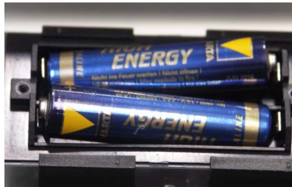
Fig. 6-140: Change the batteries, making sure the poling is correct!
