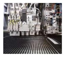
an option consisting of two lower blades, placed at right angles to each other, and two independent upper blades, again at right angles, of the same length, which are movable and equipped with blankholders. This shear can make cuts of any length, in accordance with the instructions contained in the program, and thus creates an extremely compact highperformance multifunction system for even more innovative factory sheet metal handling logistics.
