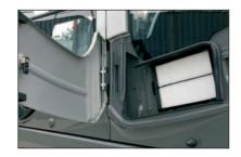
The fresh air filter for the air conditioner is relocated to cab door side from conventional location behind the operator seat. This allows easy cleaning and replacement of the fresh air filter, like the air circulation filter inside the cab.
