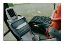
The colour LCD monitor, located in the cab, indicates coolant temperature, fuel level, and maintenance data. It also allows one-touch adjustment of the attachment. The display can also be adjusted to day or night shift.
