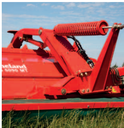
The Kverneland Taarup BX-Belt system, with individual break back of each rear mower.
