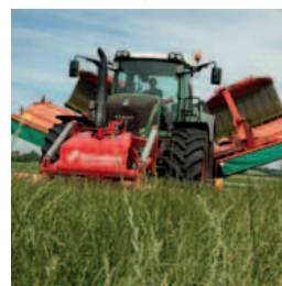
Lift of all mower units for headland turns.
