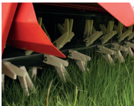
Rigid nylon tines provide aggressive conditioning.
