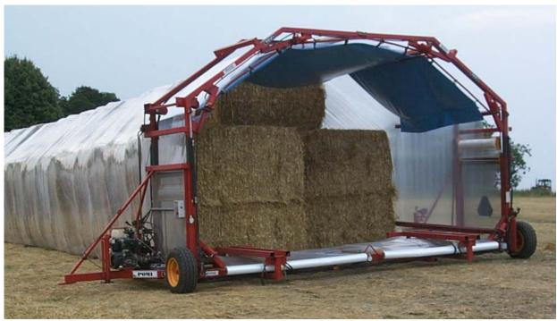
The Wrap 5 wrapper is designed according to a new concept. The machine wraps a tube of foil in which the bales are positioned with a loading unit. A large stack can be wrapped with a light machine, easy to handle. Wrap 5 is made primarily for wrapping of big straw bales, it can however also be used for wrapping all other types of rectangular bales and round bales size 1,25 m and 1,8 m.
